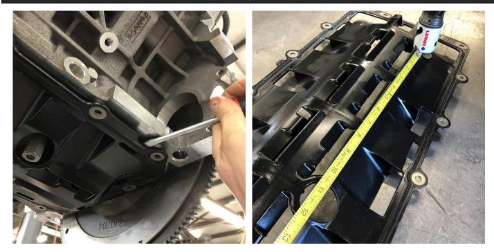
Remove the stock oil pan, oil pick-up, and windage tray. The locating pins on the factory Coyote windage tray will need to be removed. These pins aid in production assembly of the engine but are not required for this installation. To use a front sump pick-up, it's necessary to make a new hole in the windage tray 12 inches forward of the existing hole using a 1.25" hole saw or snips.
