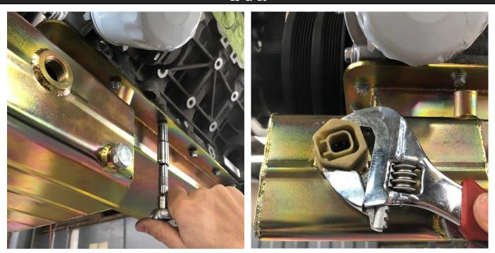
Remove the 4 temporary screws and install the oil pan tightening in an alternating pattern. Torque to 10 NM plus 45 degrees. The oil level sensor can then be reinstalled into the new pan.
