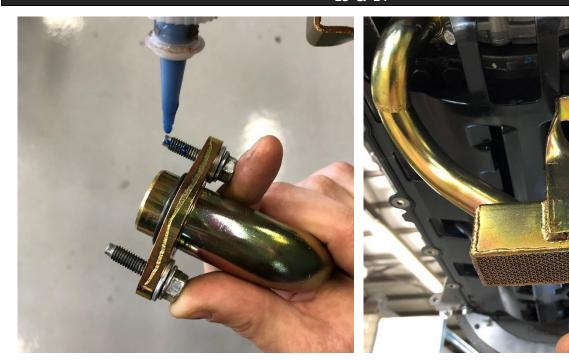
Using threadlocker, install the pick-up as shown and tighten all 3 bolts to 10 NM plus a 45 degree turn.
