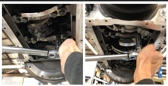
Torque both main cap screws to 65 NM.
