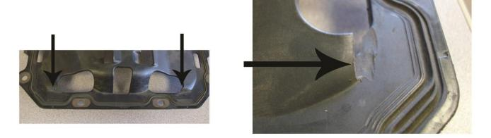
At the rear of the windage tray, 2 areas need to be ground for clearance to the new oil pan flange. The new oil pan and the tray should be checked so that they sit flat against one another.
