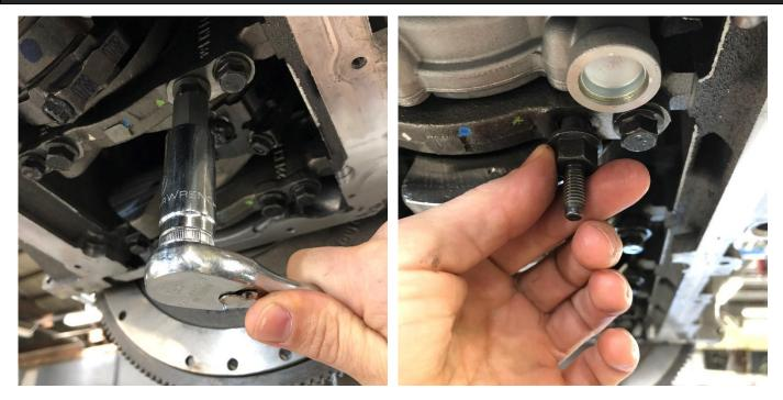
Remove the stud extension and cap screw from the rear of the block and reposition it into the front of the block. The cap screw at the front will replace the screw at the rear.
